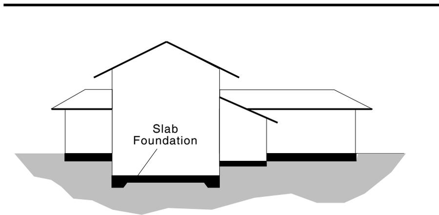
**Figure 4—Slab foundations.** *If your house was built on a concrete slab, it is probably bolted to its foundation.*
